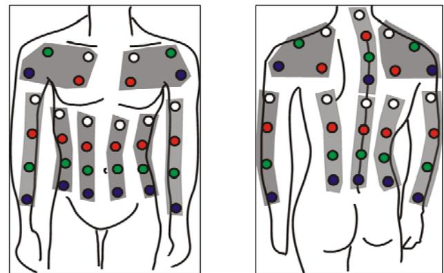
**Figure 1. Upper panel: photos of tactile jacket with outer lining (left) and inner lining containing electronics and wires (right). Lower panels: distribution of vibrotactile actuators on front (left) and back (right) of a torso. The actuators are represented by the colored circles and are grouped into 16 segments each containing four actuators.**
